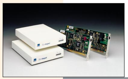
3Com Impact ISDN external digital modems and ISA adapters are easy to install and use, and give you the fastest dial-up network access at speeds of up to 128 Kbps.
